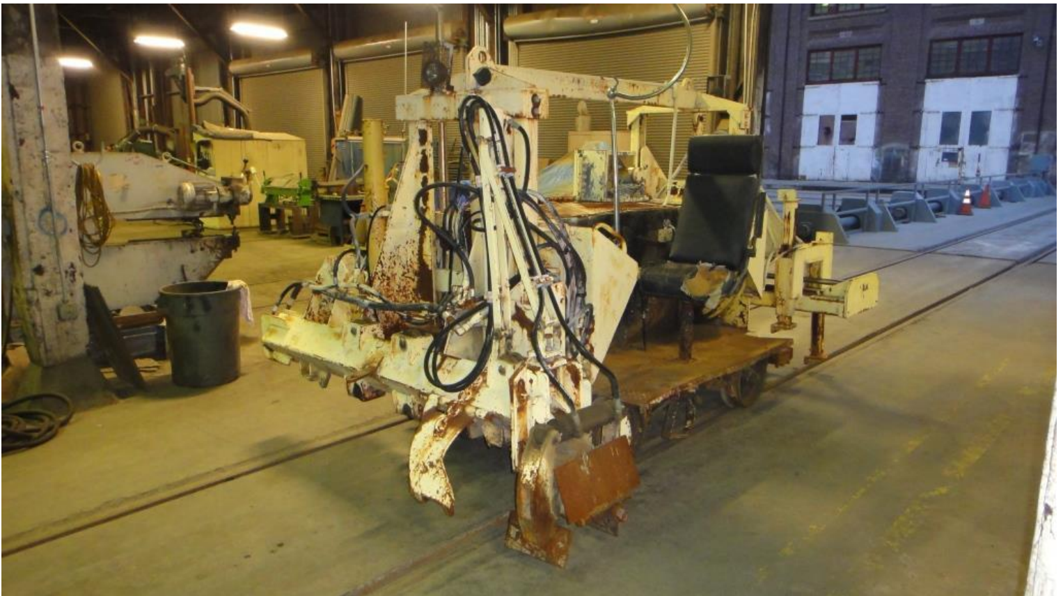
Safe and sound inside the Boiler Shop, the tie-exchanger may not look like much but, it's got a new engine and hydraulic system. It's in better shape than it looks. Most importantly, it will improve our productivity 10 fold.
